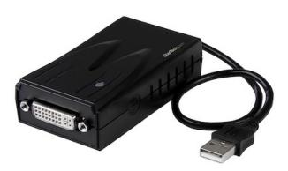
The USB2DVI USB DVI Multi Monitor External Video Adapter turns an available USB 2.0 port into an external video card DVI port - providing high quality dual-display or multi-monitor capability that can be used in a variety of laptop or desktop applications to increase your productivity.
