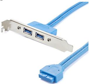
The USB3SPLATE 2-Port USB 3.2 Gen 1 A Slot Plate converts the USB pins on the USB 3.2 Gen 1 motherboard header to 2 standard USB 3.2 Gen 1 A-type ports. The plate can be mounted on the rear panel of a computer case, adding two USB 3.2 Gen 1 A female ports for simple connection to USB peripheral devices.
