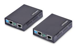
Extend a network over VDSL2, using Cat5e (or better) UTP Cabling or Single-Pair (or better) Telephone Wire at distances up to 0.6mi (1km).
